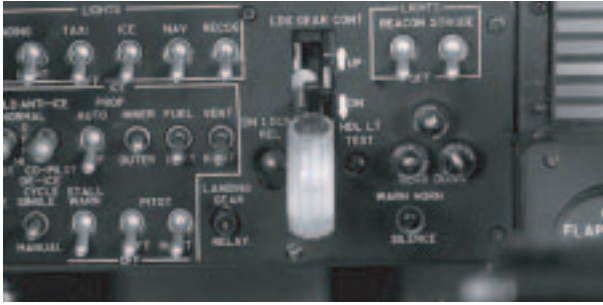
PRIOR TO BB-453 (SUBSEQUENT MODELS HAD THE GEAR DOWN INDICATOR LIGHTS IN A CUBE ARRANGEMENT)
