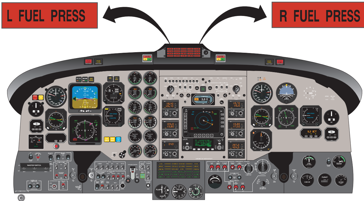
Figure 5-4. Fuel Pressure Warning Lights
