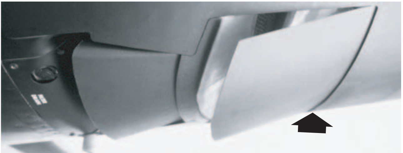
INERTIAL VANE BYPASS DOOR EXTENDED
