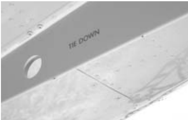
97. VENTRAL FIN DRAIN HOLES—CLEAR 98. TIEDOWN—REMOVE
