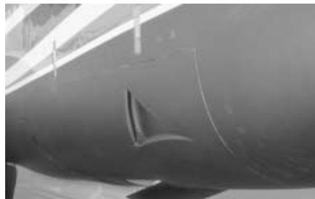
35. GENERATOR COOLING INLET—CLEAR
