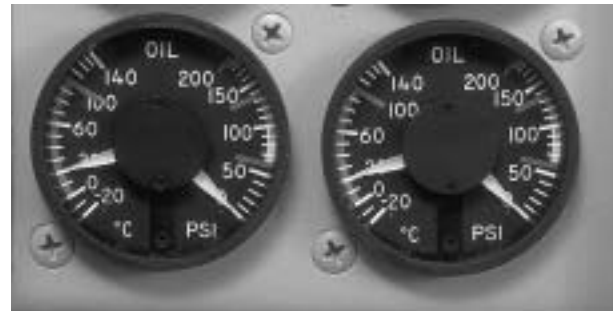
Figure 7-6. Oil Pressure/Temperature Gages
