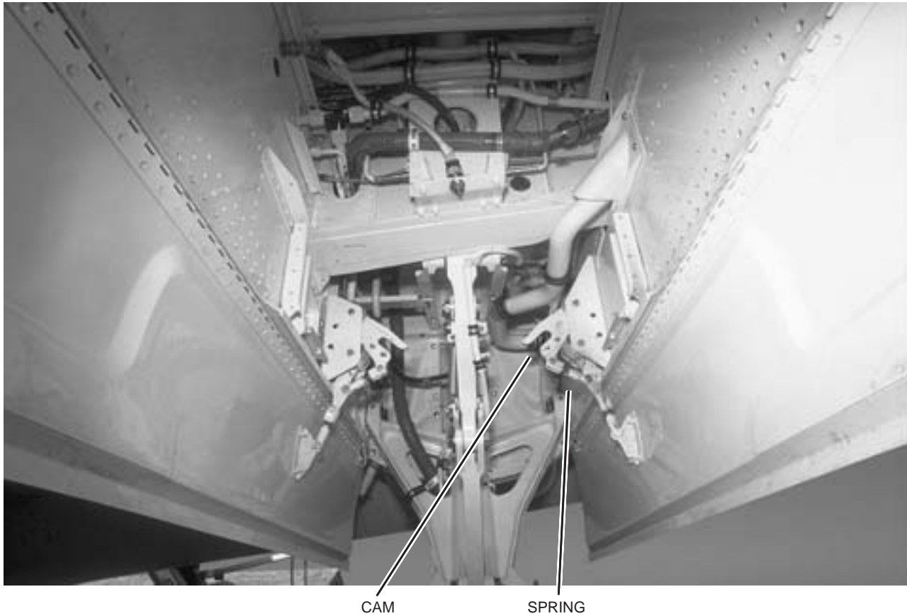
Figure 14-17. Main Gear Door Mechanism (Standard Gear)
