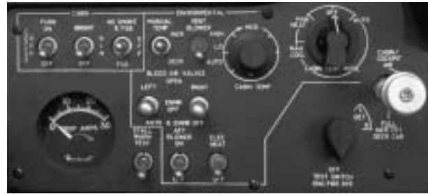
Figure 1-5. Cabin Lights Control Switch (BB-1439, 1444 and After)
