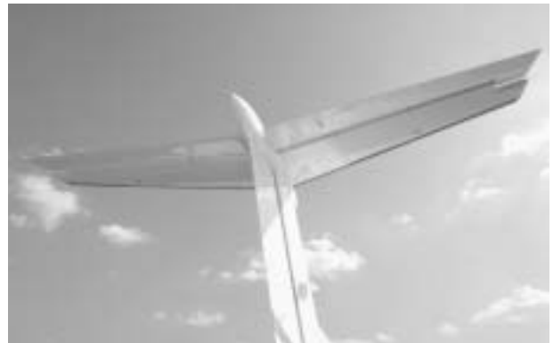
108. ELEVATOR, ELEVATOR TAB, STATIC WICKS (3 EACH SIDE)—CHECKED
