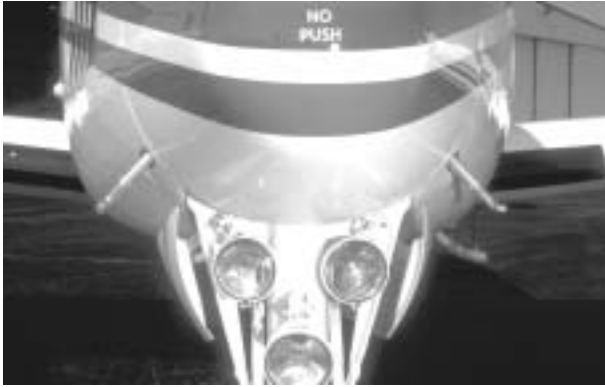
51. PITOT MASTS—COVER REMOVED, CLEAR
