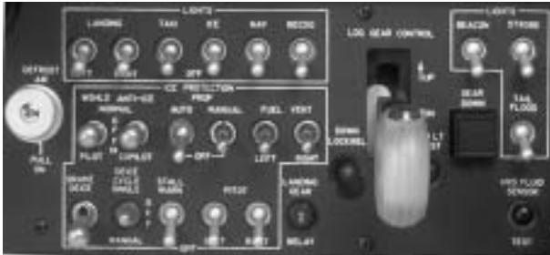
Figure 1-6. Exterior Lights Control Switches
