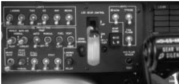
Figure 3-3. Pilot's Right Subpanel
