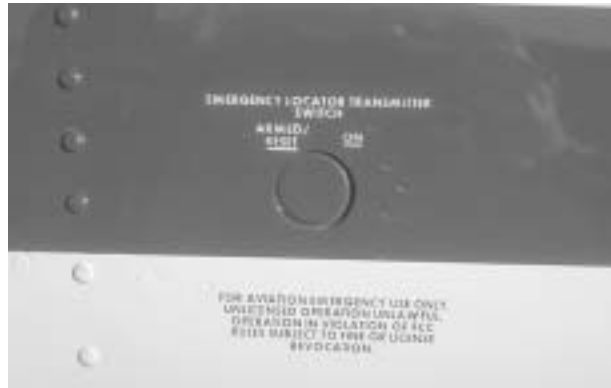
103. ELT AFT ARMING SWITCH (PRIOR TO BB-1510)— ARMED
