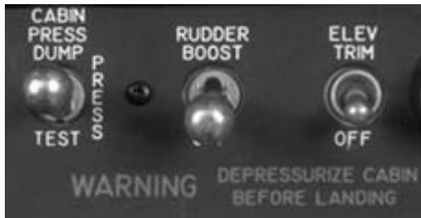
Figure 12-9. CABIN PRESSure Switch
