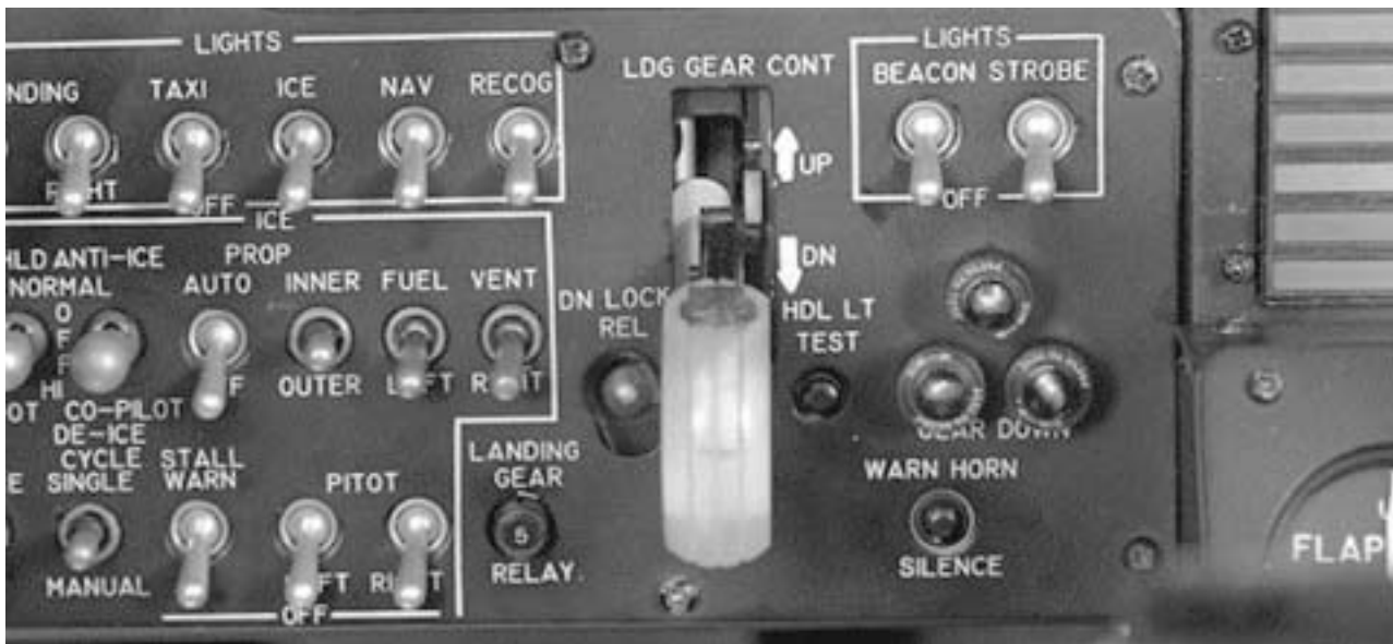
Figure 14-10. Normal Landing Gear Operation
