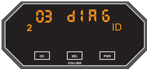
IND-42C SELF-TEST DISPLAY 03 (TRANSMITTER) FAULT FOUND
