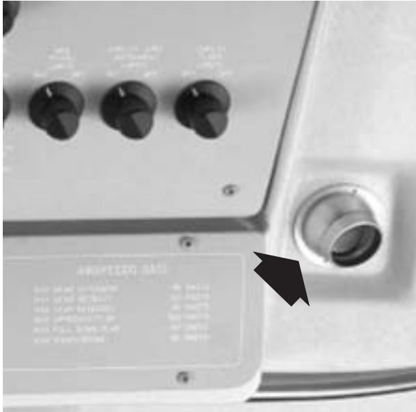
Figure 11-5. Cockpit “Eyeball” Outlets
