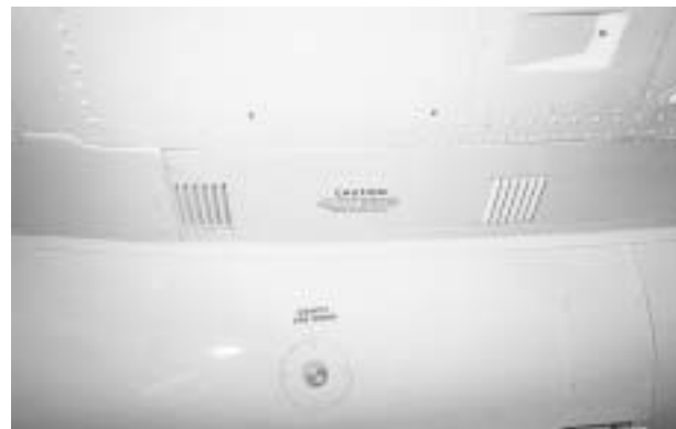
8. INVERTER COOLING LOUVERS—CHECK
