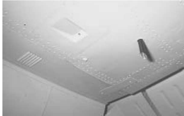
18. RAM SCOOP FUEL VENT AND HEATED FUEL VENT—CLEAR
