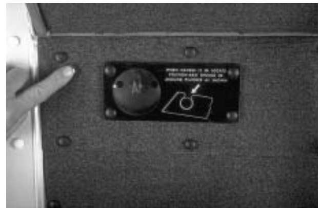
Figure 1-29. Placard and Inspection Port
