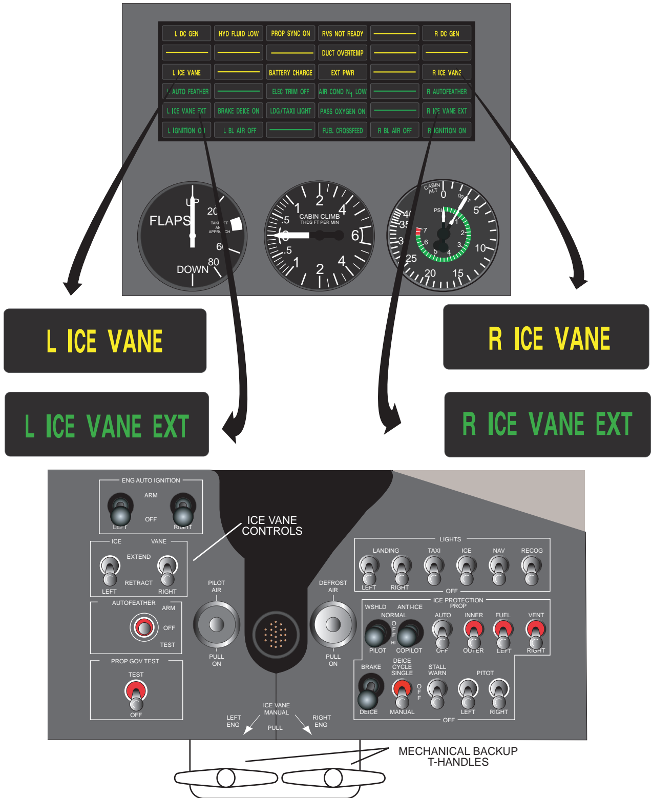
Figure 10-12. Powerplant Intake Ice Protection (Prior to BB-1444, Except BB-1439)
