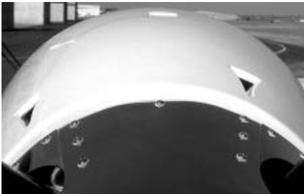
29. NACELLE COOLING RAM AIR INLETS—CLEAR
