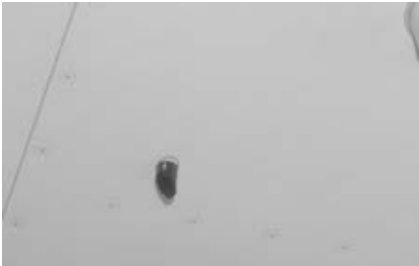
69. BATTERY BOX DRAIN—CLEAR
