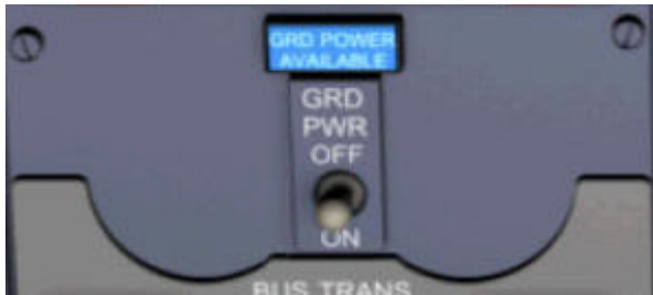
Figure 11 - Ground Power Switch
