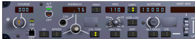
Figure 65 - MCP setup for LVL CHG descent at Mach .76
