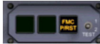
Figure 51 - FMC Annunciator on Main Panel
