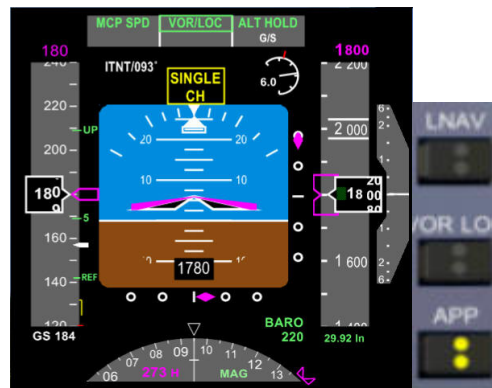
Figure 72 - Intercepting Glideslope - Approach mode armed, single channel
