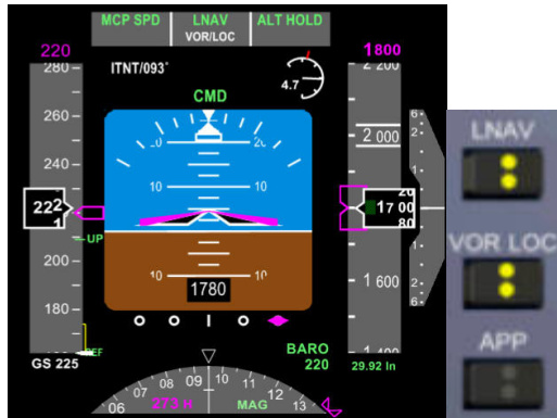
Figure 71 - 1800 feet, 220 knots, Localizer alive and Armed
