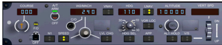
Figure 67 - MCP setup for deceleration at 10000.
