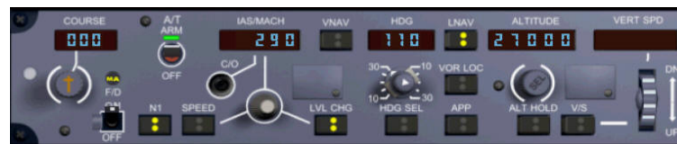
Figure 60 - MCP setup for LVL CHG climb
