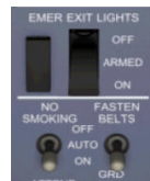
Figure 16 - Exit and Signs
