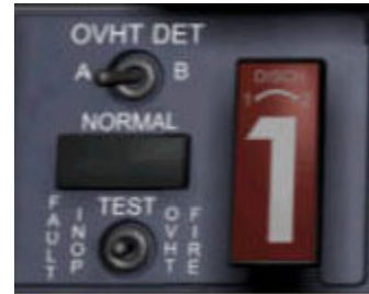
Figure 12 - Overheat Detector Test Switch
