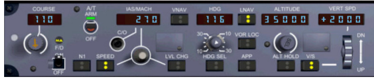
Figure 47 - Mode Control Panel
