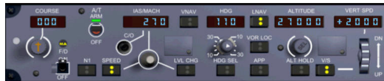
Figure 58 - MCP setup for VS climb
